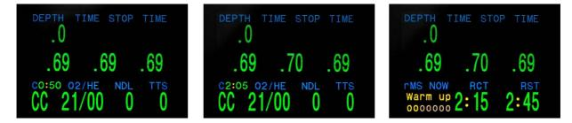
So this will become a new rule when using the scrubber monitoring system: always pre-breath until you have at least 45 minutes CYCLE time (green): this means that the scrubber is
