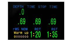
With only the temperature info at the inlet of the scrubber, the system has already received enough data to predict a minimum remaining time. You can see on the info screen that the warming up of the first zone in the scrubber has started: the color changed to yellow.
