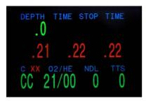
The two red XX show you that there is no communication with either of the temp probes. If communication with one of the temperature probes is successful, you see:
