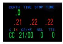
This tells you that the exhale scrubber communicates with the system, but there is no communication with the temp probe of the inhale scrubber.
