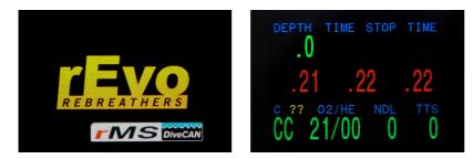
If you don't see the C ??, then the scrubber monitoring system is not activated. To activate the system, go to System Setup+, where you will find a new page 'rMS Setup'
