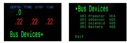
A right push on Bus Devices+ will show you all the devices connected to the CAN bus, and the software version they are using. This screen allows you to easy identify if one of the devices is missing, and if you are using the correct software in each device.
