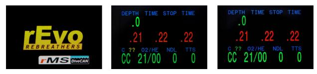
If you don't see 'C ??' this means that your temperature probes are switched off in the 'rMS Setup'. Go to the setup menu and change the setting of the temp probes to 'on'. Switching 'off' the temperature probes can be done when diving on the dual radial scrubbers, or when using classic non-rMS axial scrubbers.
