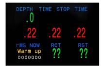
This screen shows that the unit is ready for warm up, but none of the 7 zone's in the scrubber have started to become active (they are all grey) so no prediction can be made for RCT or RST
