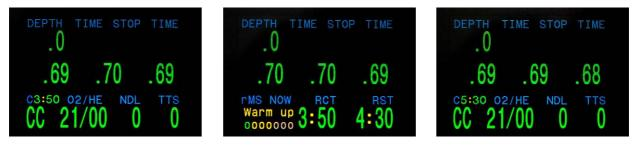
Also on the main screen there is an indication if the scrubber if fully ready or not: as long as the warming up is not yet finished, the colon between the C and the number is yellow, and only when the scrubber is fully warmed and ready, the colon becomes green, and full information of the total scrubber can be used to predict the cycle and scrubber times.
