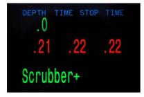
This is also a new menu for the scrubber monitoring system, that gives you information on the remaining scrubber times, and on the temperatures inside the scrubber A right pushes give you:
