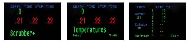
You notice that the temperatures of the first scrubber, the top scrubber, are indicated (temp 1 to 4), but that there is no indication of temperature 5 to 8: the sensors of the temperature probe in the inhale scrubber.
