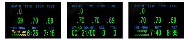
From this point on, and in dive mode, the minimum remaining cycle and scrubber time of the dive is logged, while at the same time the actual RCT/RST is shown on the main screen and the extra info screen.
